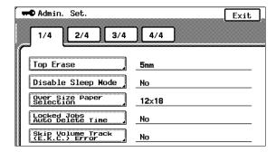
**6** Using the keypad, type in the desired length of time.
